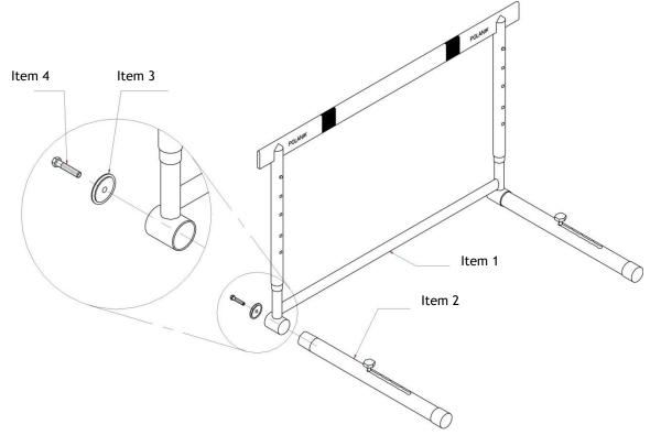
The main goal of the hurdle collapsible construction is to assure easy and cheap transport. Note that once you screw the feet down, the hurdle is practically non-dismountable. Therefore we <u>do not</u> recommend unscrewing the hurdle feet during idle periods. Removing the feet without proper tools can cause serious hurdle damages which Polanik shall not be liable for.
