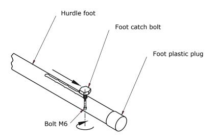
d) remove the foot catch bolt and the spring from the counterweight,
